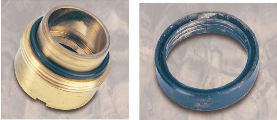
Figure 3.1 the Wear in Gland and Seal which results from Excessive Side Loading
