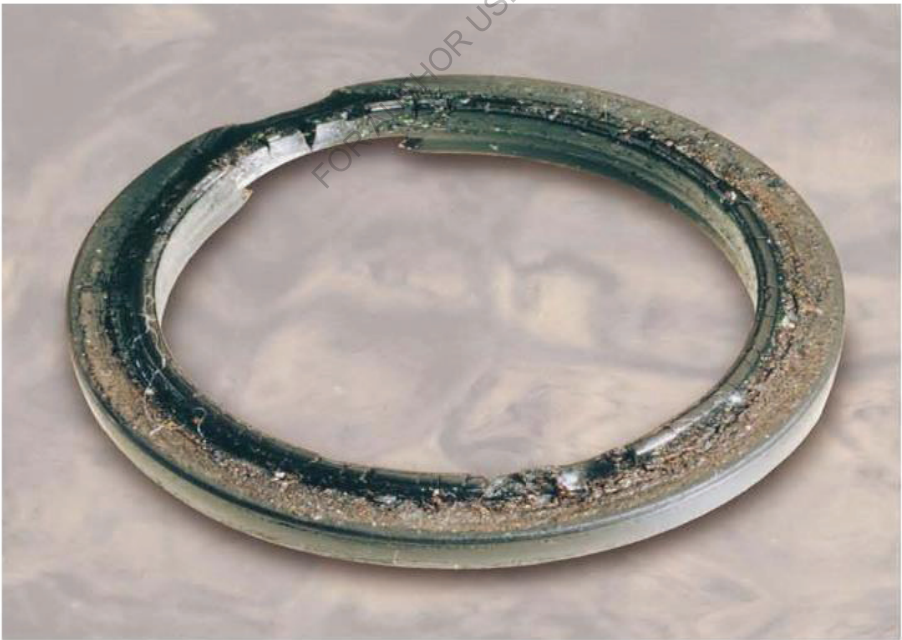
Figure 3.3 The Cracked Outer Sealing Lip of Wiper Seal which displays Damage caused by Excessive Heat
