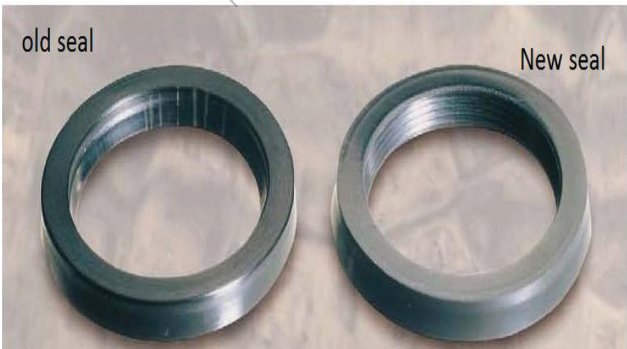
Figure 3.2 the Contamination Damage in Rod Seal
