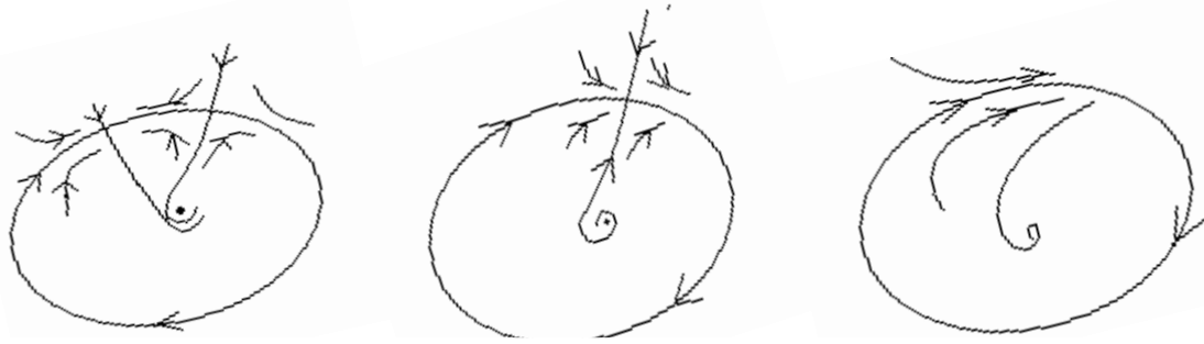
Figure (10) A saddle node occurring on a closed curve leads to global bifurcation.
